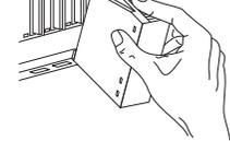
③ Secure the module with an additional screw (M3 x 12) to the base unit if large vibration is expected. This screw is not supplied with the module.
